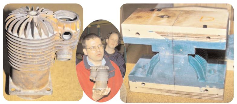
Above center is pattern maker guru **Gary Martin** holding an antique engine (shown in detail at upper left) for which he is making the required numerous patterns - one of which is shown at upper right. Gary explained some of the vagaries of making patterns for complicated machines like this.
