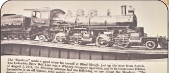
of August 1, 1911, the Mornin Mar a Whitney Company operation, and in its Centennial Edition locomotive is an oil burner; total weight of the engine and tender 121k tons, 65 tons on the drivers, and is especial waight of the engine. This locomotive has proven very satisfacany delay to the logging operation even though it negotiated, at a maximum, 26 degree curves and 8 per cent grades for three months. (B. H. Ward)
