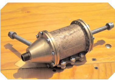
**Bill Mitchell pauses** his work long enough to show the results of the casting process. He holds a casting destined to become a pneumatic break cylinder to be used on one of his railway cars. The picture at upper right shows a finished brake cylinder that he cast last year.
