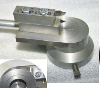
moved manually in a circle cutting a spherical shape. Tom didn't say if he used this to cut the ball handles in a quorn.
