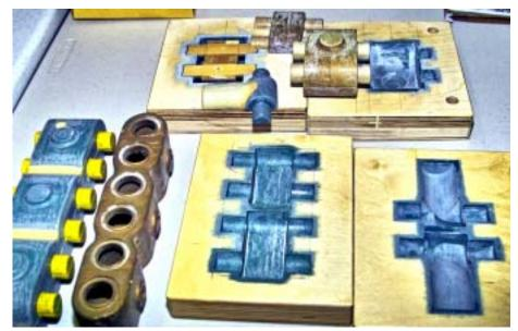
**Gary Martin** brought the molds (at left) for the 1910 Holt caterpiller tractor parts he has been contracted to make.
