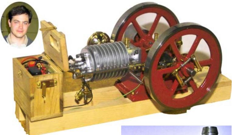
**Mike Foti** (see inset above) does it again. He constructed the Gade engine from a kit supplied by Gary Martin. This hit and miss gas engine includes a Jerry Howell ignition and was machined on a Sherline lathe. Mike expects it to be operational after a fuel tank is added.
