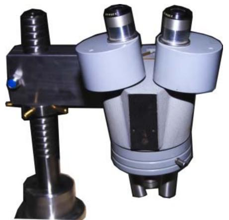
**Hal May** made an impressive stand for his microscope head shown at left. The head is able to swivel through all reasonable angles. Although not pictured, Hal also brought in one of his 3 wind up clocks designed by John Wilding.
