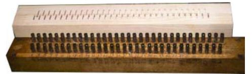
Al Pohlpeter is constructing a tracker bar (shown partly constructed at left, upper) based on the original (left, lower) for a Wurlitzer Automatic Harp. Al says there are only 20 of these harps in existence.
